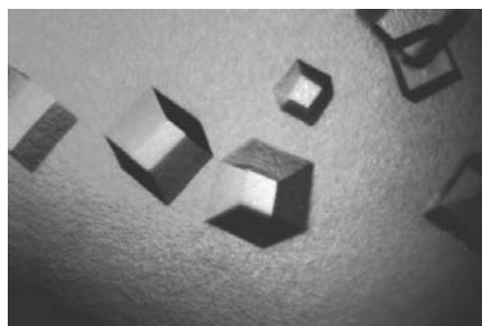
Figure 1 Crystals of GlpK as grown by the hanging-drop method. The average dimensions of these crystals were 0.3 \times 0.3 \times 0.3 mm.
